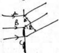
path diff. b/w secondary waves starting from A & C is  $AC \sin \theta = (a+b) \sin \theta$
