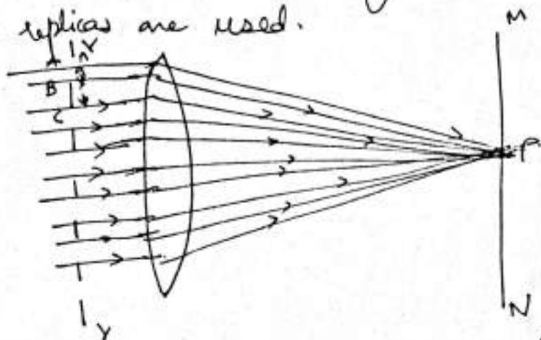
All the secondary waves travelling in the same direction as that of the incident light will come to focus at the point P on the screen.
