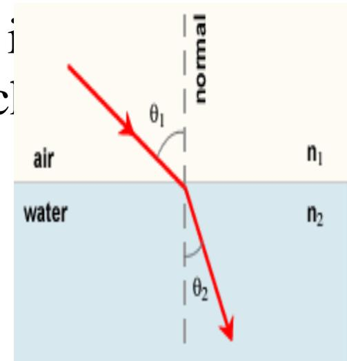
$\theta_1$  is the incident angle between the light beam and the normal (normal is  $90^\circ$  to the interface between two materials)
