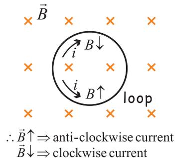
However, even in the *absence* of the loop (so that there is no induced current), the induced E-field will still accompany a change in magnetic flux.
