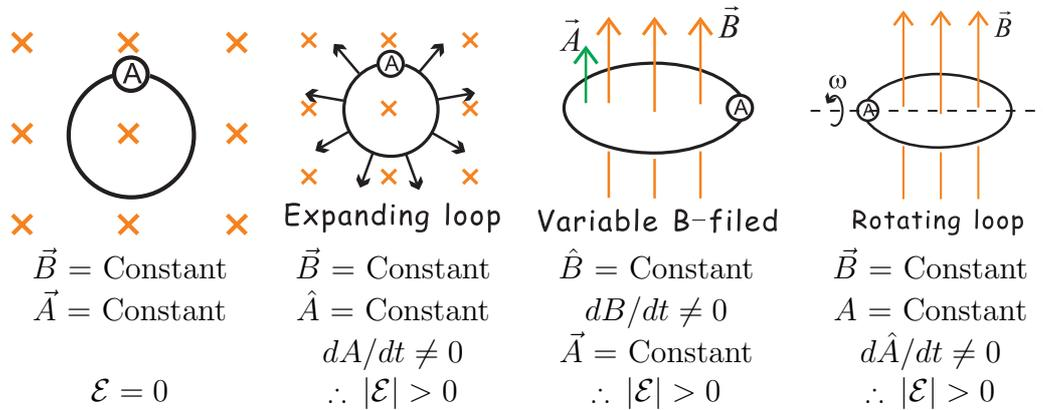
**Note :** The *induced emf* drives a current throughout the circuit, similar to the function of a *battery*. However, the difference here is that the induced emf is *distributed throughout the circuit*. The consequence is that *we cannot define a potential difference between any two points in the circuit*.
