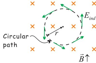
The induced E-field only has tangential components. (i.e. radial E-field = 0)
